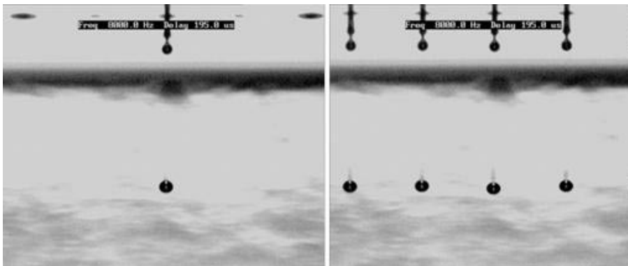
Figure 4: Single jet firing vs. all jets firing — showing minimal cross-talk
