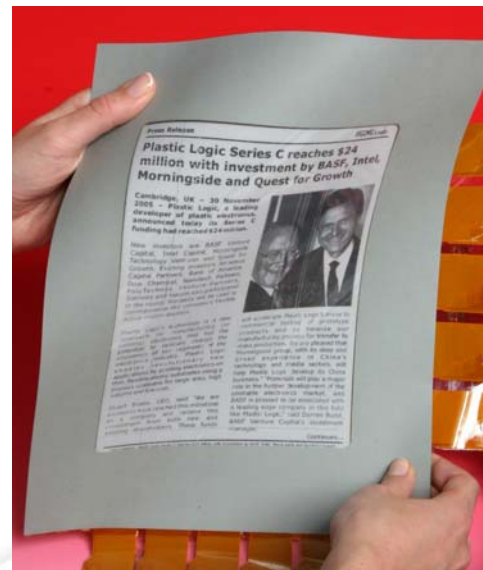
Plastic Logic flexible backplane December 2005
